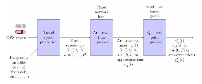
Figure 1: From GPS vehicle traces to quickest path queries proposed in [2]
